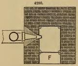
from 20 to 25 in. high above, and from 8 to 14 in. deep below the tuyere. The sides are formed of thick cast-iron plates, and the bottom of beaten clay or slag; or in the more modern hearths, of iron, cast hollow, so as to allow of their being kept cool by a stream of water circulating through them.
